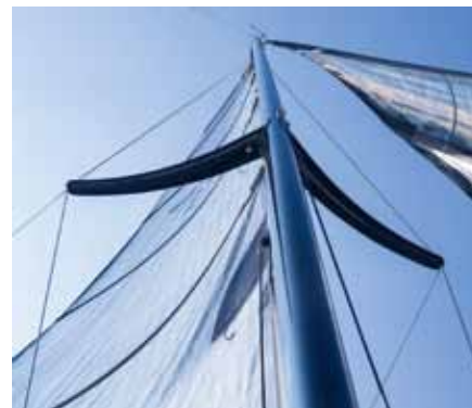
Curved spreaders eliminate interference with the vertically battened self-tacking jib
