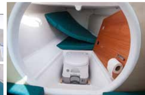
ABOVE Through the hole to the heads. The ring frame between the beams has to be massively strong.
