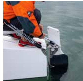
Open-backed rudder stocks allow the blades to be moved vertically – and, importantly, to kick up on impact
