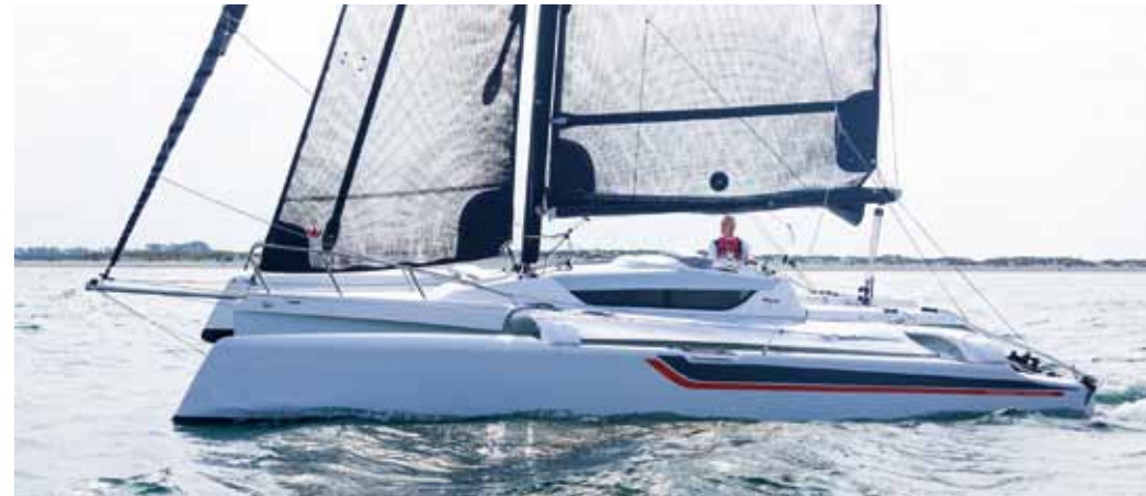
The 25 is the first Dragonfly to sport reverse rake on the bows of the floats. It's functional as well as fashionable
