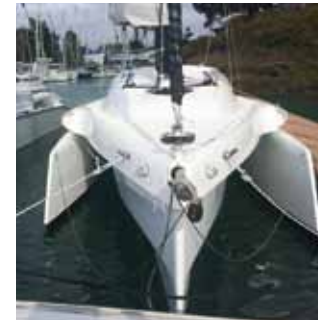
Narrow beam when folded, combined with a weight of just over a ton, simplifies trailing and marina berthing
