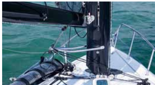
Controlling rotation: the bottom line limits the mast's maximum rotation and the top one determines its angle in relation to the boom
