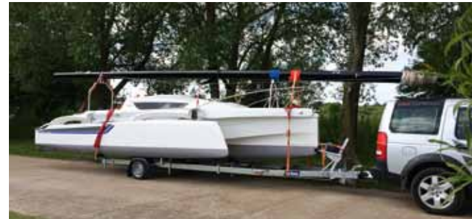
Narrow beam when folded, combined with a weight of just over a ton, simplifies trailing and marina berthing
