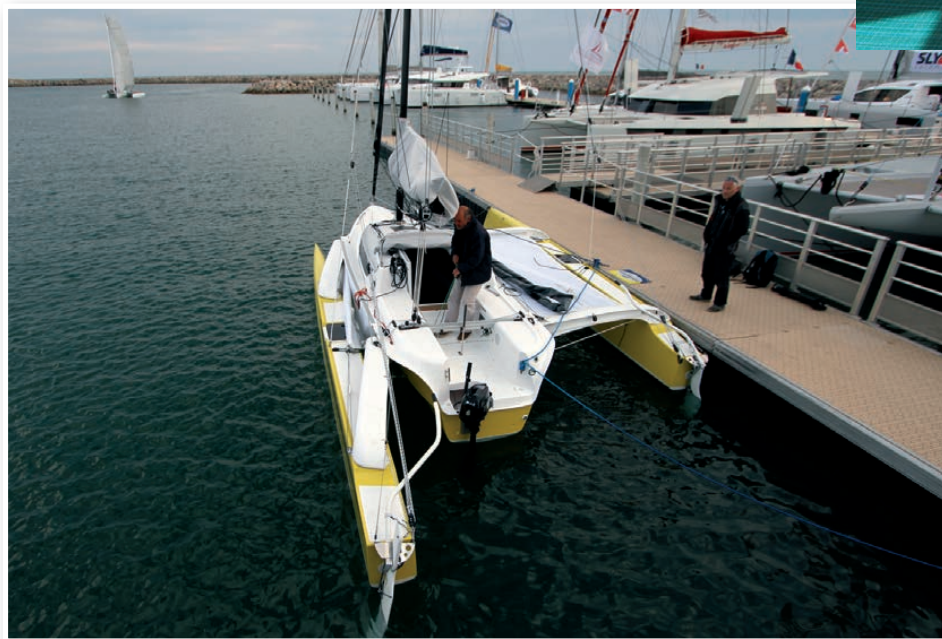
Dragonfly: Folding trimarans which, once in port, slide into a monohull slip, or fit onto a road trailer. Clever!
