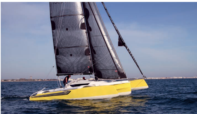
↑ Dragonfly: At first glance, you notice the inverted bows of the floats and the crossed beams... classy!
