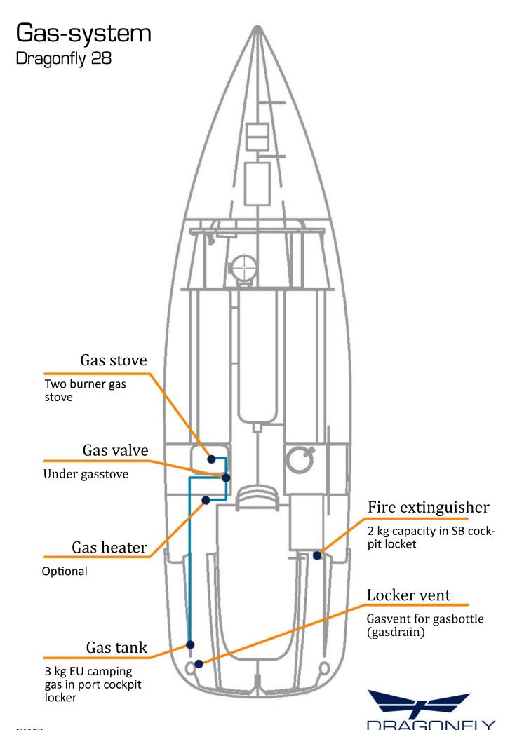
**VERY IMPORTANT**: Never use the gas stove or -oven with closed cabin doors and hatches and make sure to have airflow and ventilation in the main cabin when using the gas systems.
